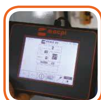
Programmatore Touch screen 5,7" removibile. 5,7" removable touch screen programmer
