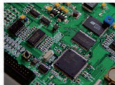
High speed CPU control circuit
