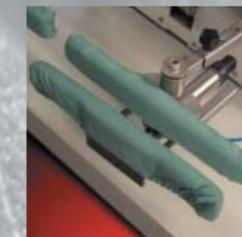
*the trouser leg tensioning clamps can be adjusted in various position as to better fit the different trousers styles*
