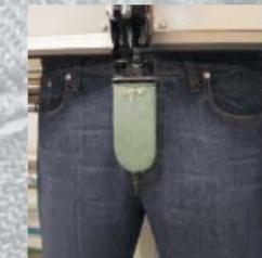
*the front waistband-fly locking keeps the garment in the correct position during the pressing cycle*
