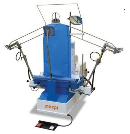
Electropneumatic steaming and blowing dummy for finishing of dry sweaters, T-shirts and polo, complete with:
