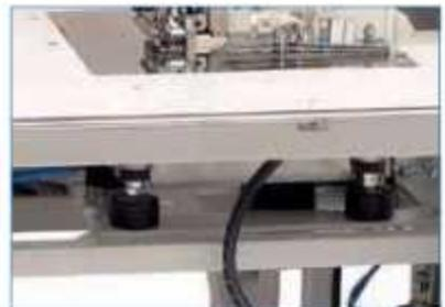
The sewing unit FX 2300-EXT is the economy version for sewing sideseams and inseams. The compact design is especially suitable for the universal use in the production of sportswear trousers. Due to the pneumatically moveable edge guide it is possible to trim the excess lengths of pocket bags.
